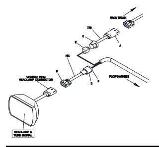
Figure 1. Ford F150 Headlight Adapter Installation G10876
